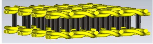
Fig. 1. Structure of the proposed electromagnetic shield
