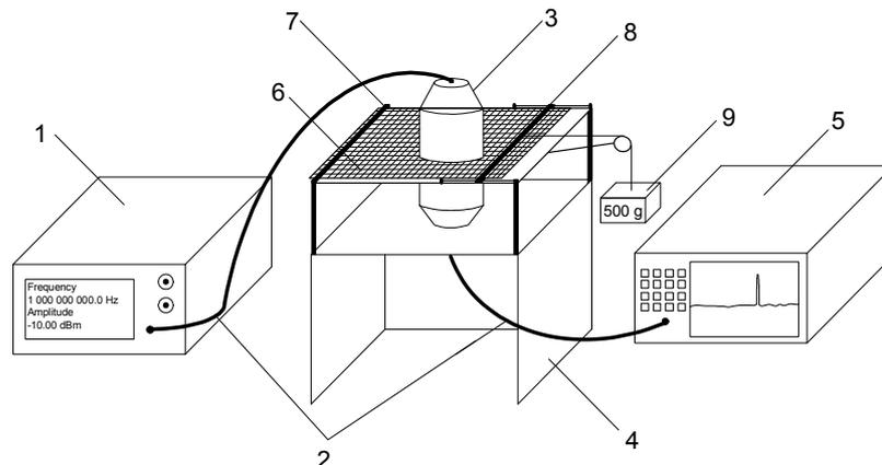
Fig. 2. SE measuring stand: 1. RF signal generator, 2. coaxial cables, 3. SE test fixture, 4. stand/holder for the test fixture, 5. spectrum analyzer, 6. tested fabric, 7. fixture, 8. mobile fixture, 9. weight.
