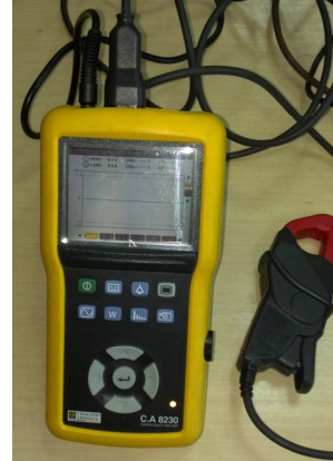
Fig.2. Power analyzers tested
