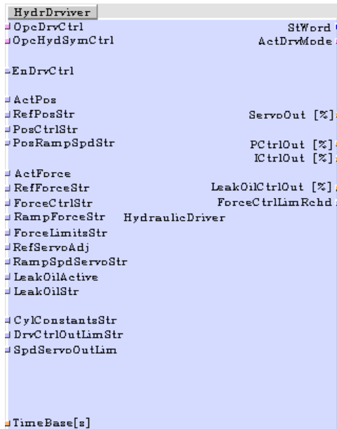
Fig. 7 Integration diagram of the new auto-adaptive driver module for hydraulic positioning in LogiCAD representation
