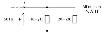
Calculate the admittance (reciprocal of impedance) of the entire circuit and the phase angle between I and V. What is the power factor of the circuit?
