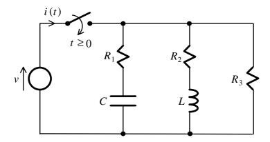
Derive an expression for i(t) as a function of time. For what values of  $R_1$ ,  $R_2$  and  $R_3$  will this current be independent of time?
