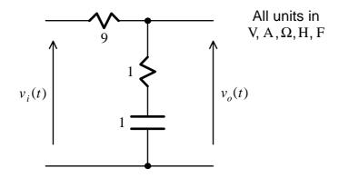
Determine  $\boldsymbol{v_o}(t)$  if  $\boldsymbol{v_i}(t)$  is given by the non-periodic signal
