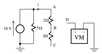
Assuming that VM does not take any current, determine the current i and the voltmeter reading when
