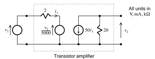
Determine the output voltage  $v_2$  of the amplifier in terms of  $v_1$ . What is the gain of the amplifier in terms of voltage magnitudes? Give your answer in dB. Determine the Thevenin's equivalent circuit of the system as seen from the output terminals.
