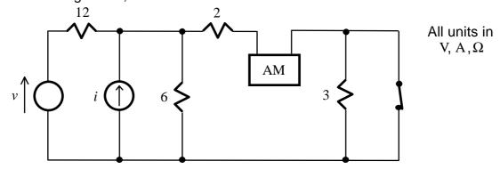
Using Norton's equivalent circuit, determine the reading when the switch is open.
