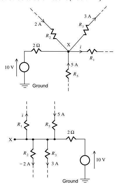
As is done in the above circuits, voltages in electrical systems are often measured with respect to a reference or ground potential. In practice, the ground will be connected to a large number of components and will run through the entire system using thick conductors. It is sometimes connected to the chassis of the system or the earth pin of the 3-pin power plug.
