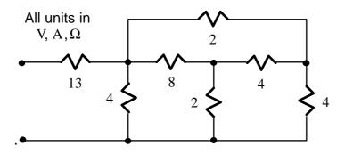
Q.5 Determine Norton's and Thevenin's equivalent circuits for the following 2-terminal network.
