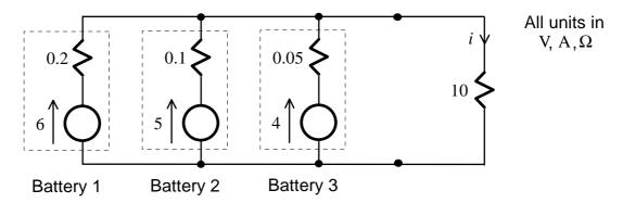
Using superposition, determine the component of the load current i due to each battery. Hence, calculate the load current.
