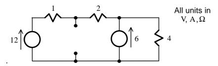
Q.4 Determine the resistor that will draw a current of 2A when connected across the two terminals of the following network.
