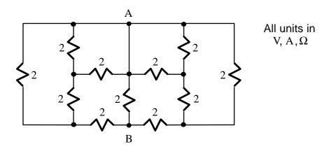
What will the result be if the outer two resistors are short-circuited?
