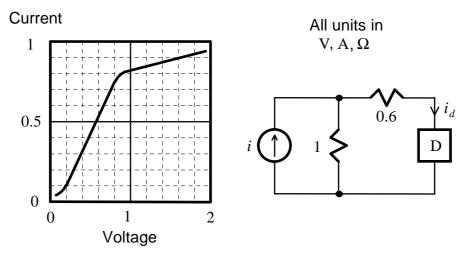
Determine the device current  $i_d$  if  $i = 1.6\,\mathrm{A}$ . At what value of i will the power dissipated in D be  $0.6\,\mathrm{W}$ ?
