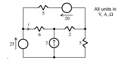
Q.3 Determine the maximum power that can be obtained from the two terminals of the following circuit.
