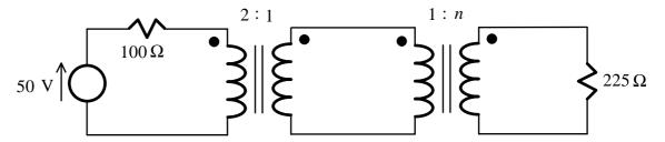
Given that maximum power is being drawn from the source, determine the turn ratio n and all the voltages and currents in the circuit.
