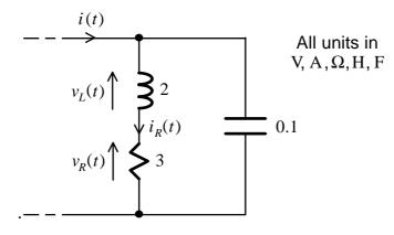
Determine  $i_R(t)$ ,  $v_L(t)$  and i(t) by using phasor analysis.
