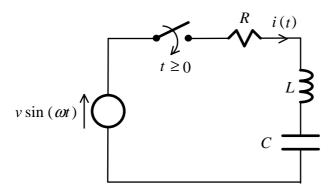
Derive the governing differential equation and initial conditions for finding the circuit current i(t) for  $t \ge 0$ . Determine the steady state current.
