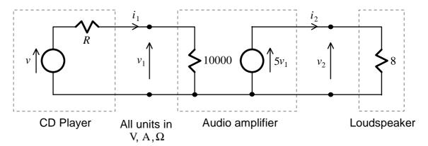
Calculate the voltage gain  $|v_2/v_1|$ , current gain  $|i_2/i_1|$  and power gain  $|(v_2i_2)/(v_1i_1)|$  of the amplifier in dB. What is the relationship between these gains? Show that these gains will be equal to one another when the load resistance is equal to input resistance of the amplifier. Do you expect this to be the case in practice?
