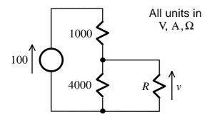
In finding v, a novice (=1st year student) may forget (okay, if it's only for this time) to include the loading effects of R. To understand these effects, determine v and the current in R when
