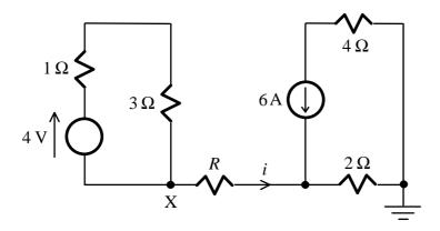
How will these be changed if the circuit is not grounded or if the circuit is grounded at Point X only?
