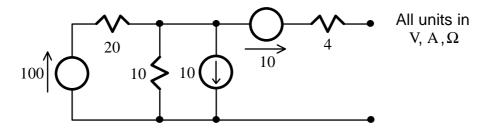
What resistor will absorb the maximum power? Calculate this power.
