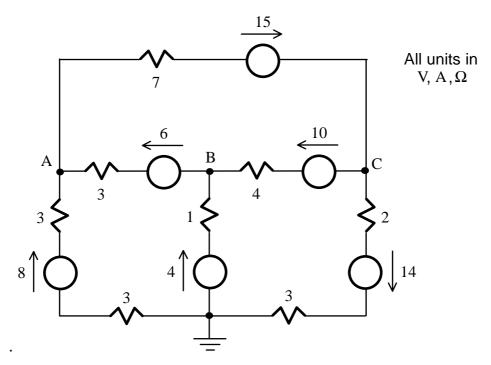
Using nodal analysis, derive the equations for obtaining the voltages of the three nodes.
