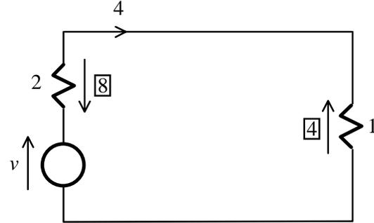
$v = 8 + 4 = 12 \text{ V}; i = 1; \text{ voltage across } 3\Omega \text{ resistor} = 3i = 3 \text{ V}$
