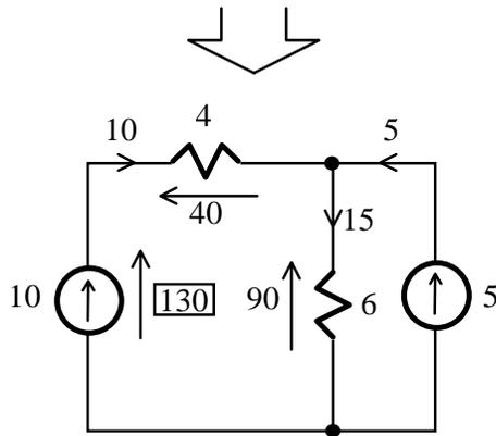
The 10A current source is supplying a power of  $(130)(10) = 1300\text{W}$ .
