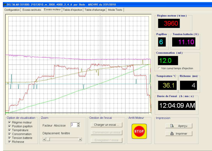
Figure 5 – The evolution of the fuel consumption slope and motor speed for different load degrees
