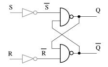
The circuit has the inputs active on logic 1. If the inverters are taken out, the circuit will have the inputs active on logic 0.
