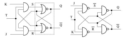
Their disadvantage is that for T=1 the circuit oscillates.
