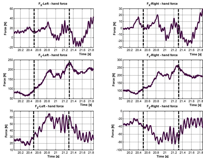
Fig. 6. Recorded data for handle reaction forces (positive values for FX [forwards], FY [vertically up], and FZ [lateral]) during On/Off controlled sitting down; the controller is operating between 20.5 and 21.3 seconds.
