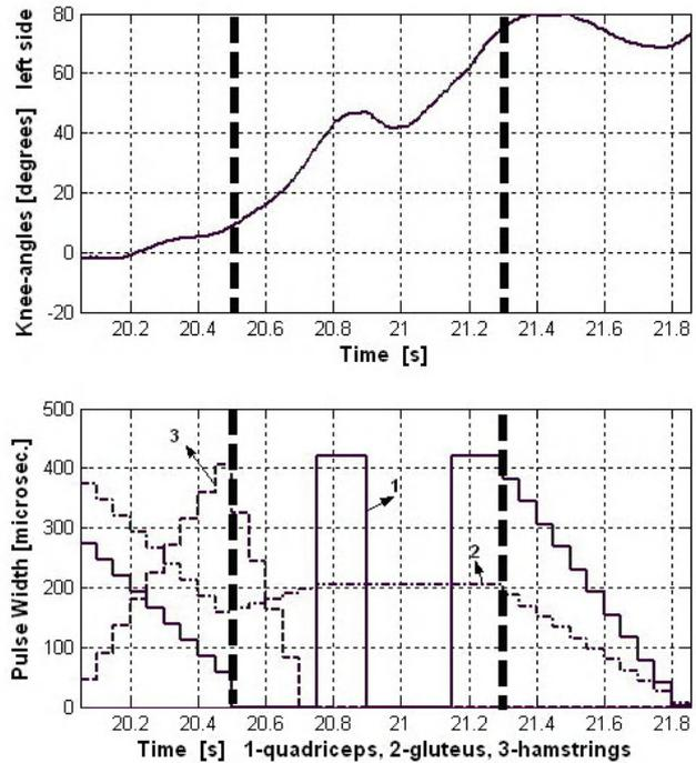
Fig. 5. Recorded data for the left side during the On/Off controlled sitting down motion task: knee angle (top plot) and stimulation pulsewidth (bottom plot) against time. The controller is operating between 20.5 and 21.3 seconds.
