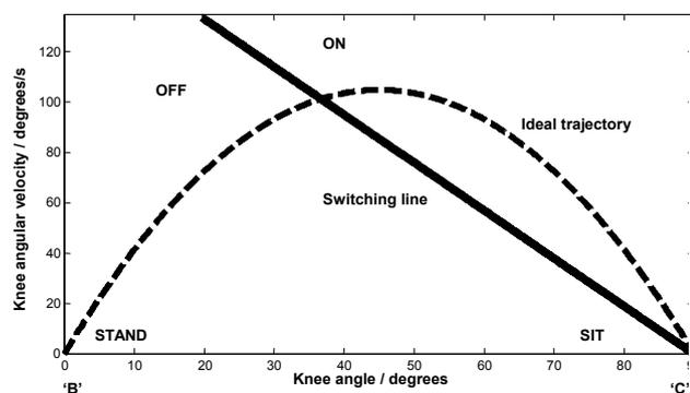
Fig. 2. State-space diagram for knee angle against knee angular velocity as for the On/Off controller (adapted from [18]). The switching line defines the On and Off regions, whereas the ideal trajectory would represent a smooth transition from standing to sitting. Points 'A', 'B' and 'C' are described in the text.
