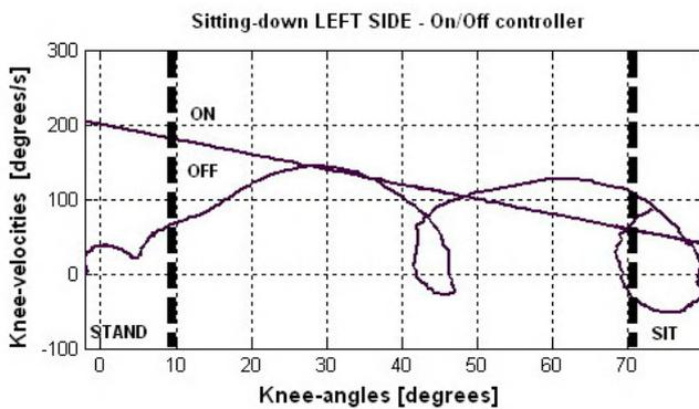
Fig. 4. Knee angle against knee angular velocity state-space trajectory using an On/Off controller to support sitting down (recorded data for the left side). The controller is defined by  $Ox = 100^\circ$ , gradient =  $-2 \text{ s}^{-1}$  and operating between  $10^\circ$  and  $70^\circ$  (c.f. solid straight line).
