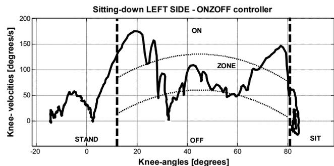
Fig. 7. Knee angle against knee angular velocity (data for the left side) in a state-space trajectory using an ONZOFF controller to support sitting down. The controller is defined by  $O_x = -10$  and  $100^\circ$ , maximum knee angular velocity =  $120^\circ \text{ s}^{-1}$ , a zone width of  $70^\circ \text{ s}^{-1}$  and operating between  $10$  and  $80^\circ$ .
