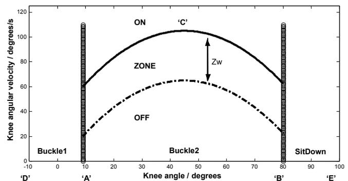
Fig. 3. State-space diagram for knee angle against knee angular velocity as for the ONZOFF controller. Points 'A' through to 'E' are described in the text.
