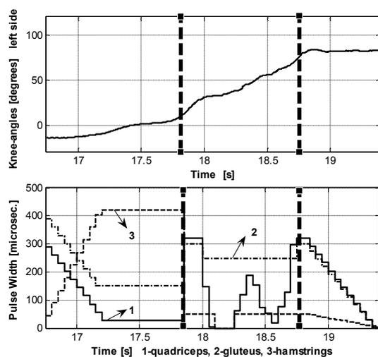
Fig. 9. Recorded data for the left side during the ONZOFF controlled sitting down motion task: knee angle (top plot) and stimulation pulsewidth (bottom plot) against time. The controller is operating between 17.8 and 18.75 seconds.
