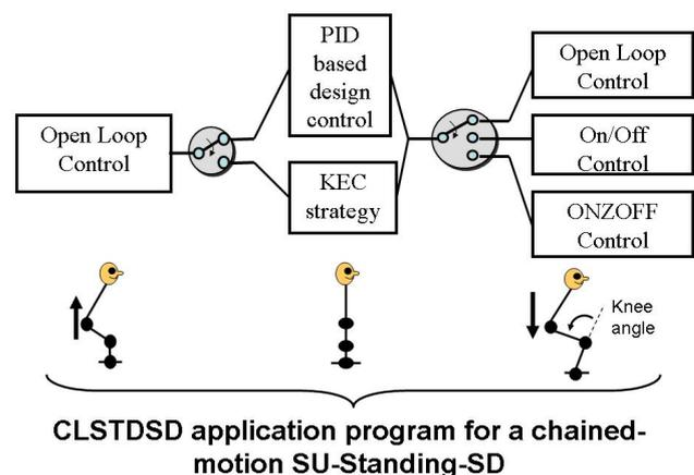
Fig. 1. Application program diagram for FES-assisted standing up (SU), standing and sitting down (SD).
