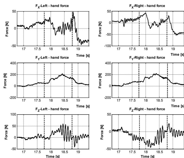
Fig. 8. Recorded data for handle reaction forces (positive values for  $F_x$  [forwards],  $F_y$  [vertically up], and  $F_z$  [lateral]) during ONZOFF controlled sitting down; the controller is operating between 17.8 and 18.75 seconds.
