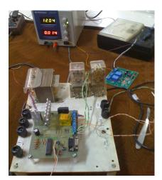
Fig. 2 – Testing scheme of control board operation.
