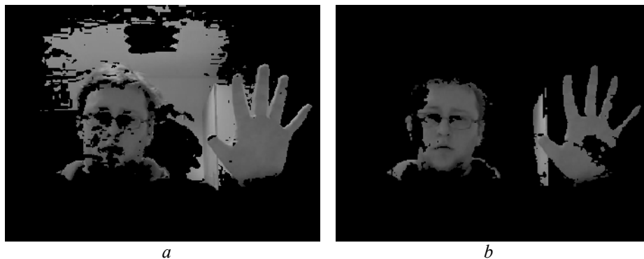
Fig. 2 – Skin detection results: a – threshold on Y -component; b – thresholds on H - and S -components.
