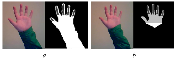
Fig. 5 – Skin detection in a non perturbed case: a – initial hand detection, b – skin segmentation result in the next frame.
